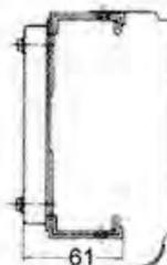
**Circuit isolating section (with Feed-In) for 60 and 100 amps**
